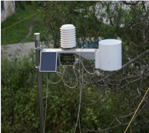
Plate 2: i-Metos automatic weather station installed in an apple orchard
